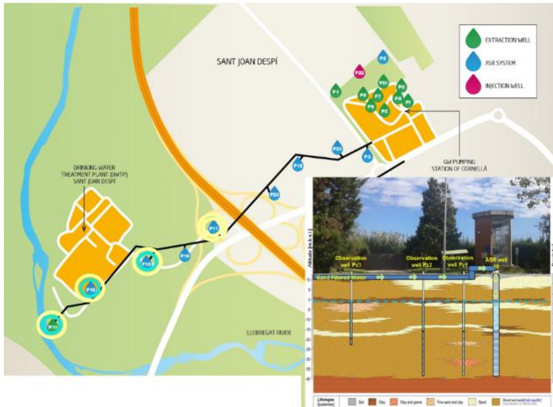
Figure 3: DS1 infrastructure (P18 deep injection MAR system)
